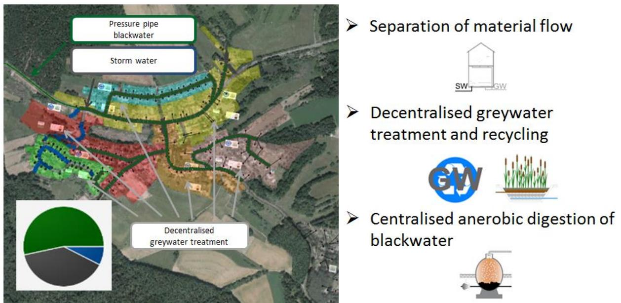
**Fig. 4.** Optimization solution with decentralised measures for the separation of material flow with separated blackwater and greywater treatment. Graphic: University of Kaiserslautern
