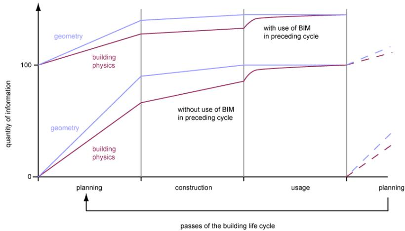
Fig. 2: Relative volume of information for building physics and geometrical survey (with and without use of a BIM)
