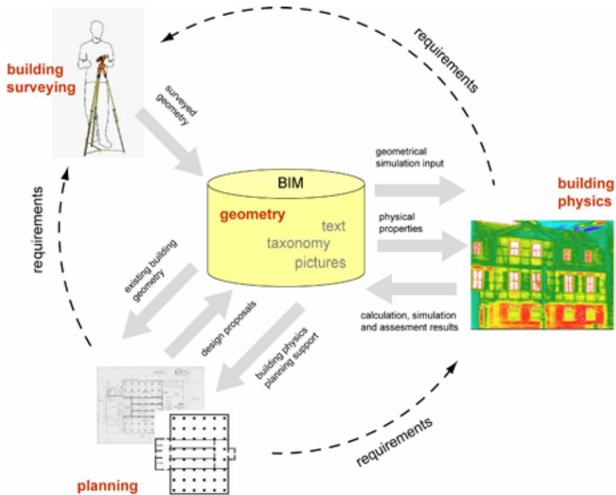
Fig. 3: Data flow between surveying, planning and simulation
