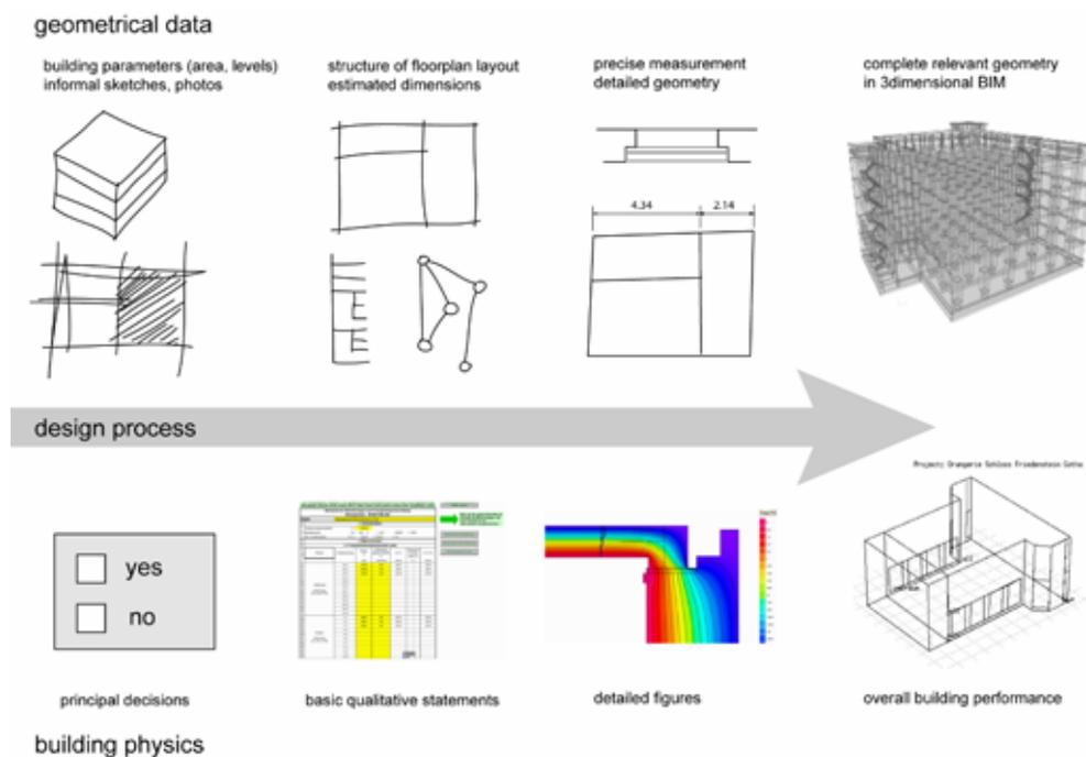
Fig. 1: Design stages showing the relevant issues of building physics and level of detail of the surveyed data
