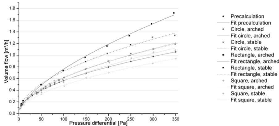
**Fig. 7:** Volume flow at stable and arched membranes
