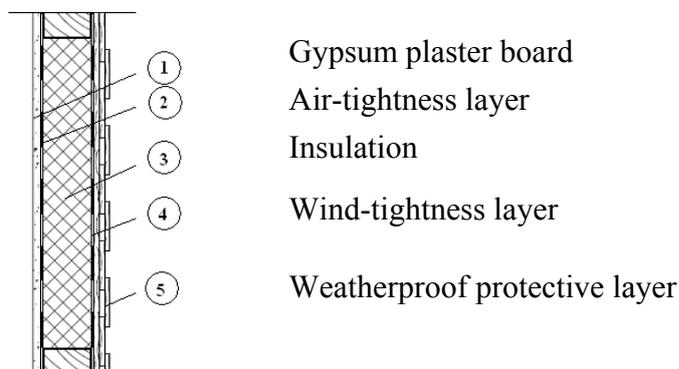
**Fig. 2:** Wood frame construction, inside left and outside right.
