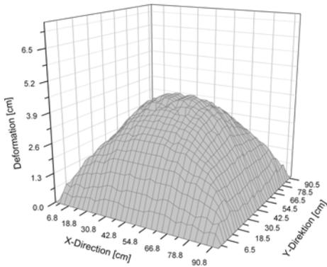
**Fig. 5:** Curvature of PE-foil under 50 Pa with a leak of 0.2 cm<sup>2</sup>
