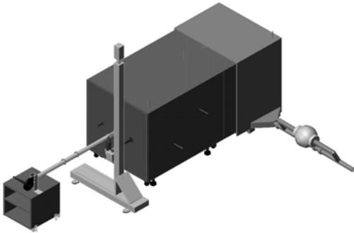
**Fig. 4:** Experimental setup for analysis of convective moisture transfer through leakages.
