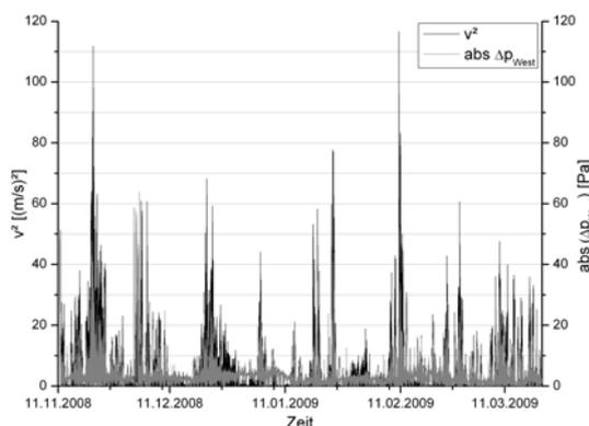
**Fig. 3:** Comparison of the wind speed to the power of two with the value of the force of pressure difference on a west facade in Weimar
