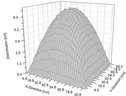
**Fig. 6:** Curvature of PE-foil under 350 Pa with a leak of 0.2 cm<sup>2</sup>
